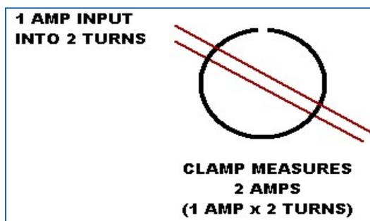
It is this principle, which enables a clamp meter to be calibrated at much higher currents than is directly available. By producing a coil with a known number of turns the input current is multiplied by the number of turns on the coil.
