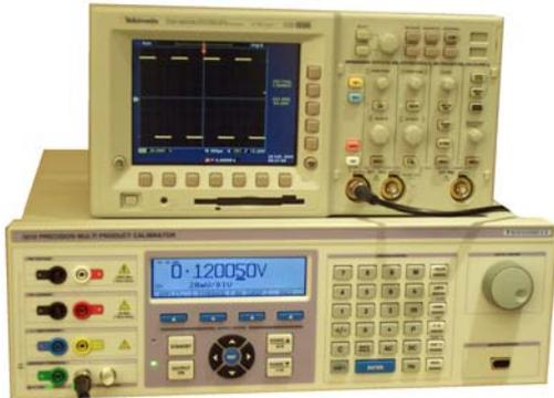
Oscilloscopes have always been an important measurement tool for the engineer. The design of oscilloscopes has evolved slowly from early instruments which were used to simply view a waveform, to oscilloscopes with calibrated ranges and graticules (grid) on the display to enable measurements to be made, up to the modern digital storage oscilloscope (DSO) which have many advanced measurement functions built in as standard.
